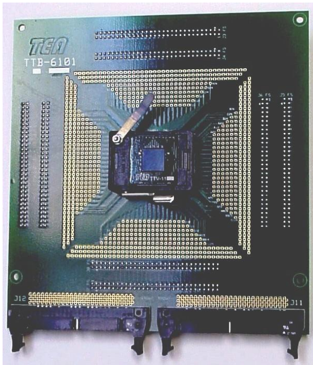
Top view showing BGA socket & ribbon cable connectors
