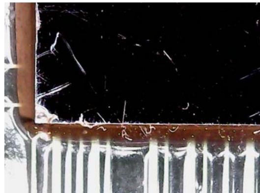
Example of chipped corner and fracture starts
