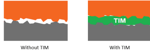
Fig. 5. Thermal interface material between interfacing surfaces
